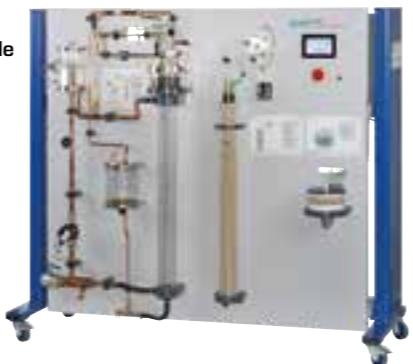
**ET 264****Geothermal energy with two-well system**
