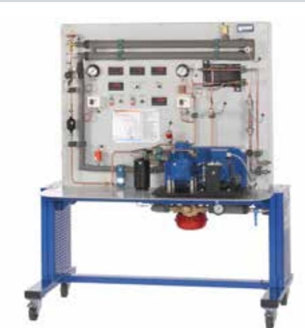
**ET 430****Refrigeration system with two-stage compression**
