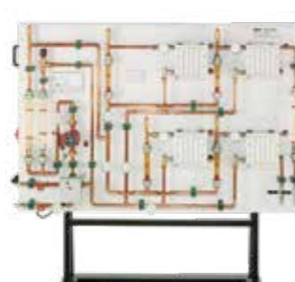
Model of a central heating system with radiators, circulating pump and four-way mixing valve
