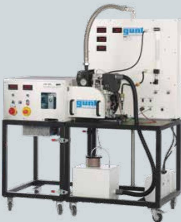
Modular test stand for single cylinder test engines CT 159, test engine CT 151 and brake unit HM 365
