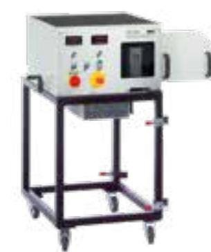
**ET 432****Behaviour of a piston compressor**
