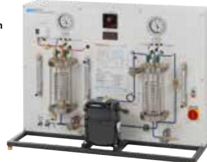
Energetic analyses of the refrigeration cycle; transparent components offer insights into the changes of state
