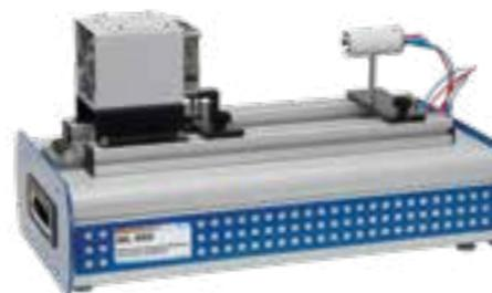
**WL 372****Radial and linear heat conduction**
