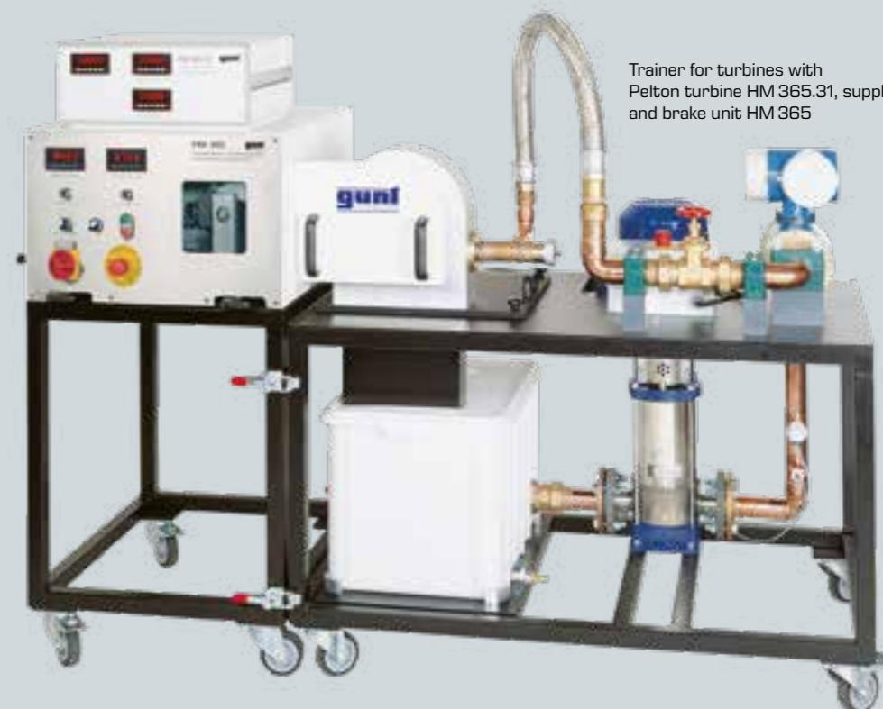
Trainer for turbines with Pelton turbine HM 365.31, supply unit HM 365.32 and brake unit HM 365
