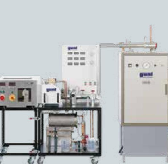
Experimental plant with two-cylinder steam engine ET 813, steam generator ET 813.01 and brake unit HM 365
