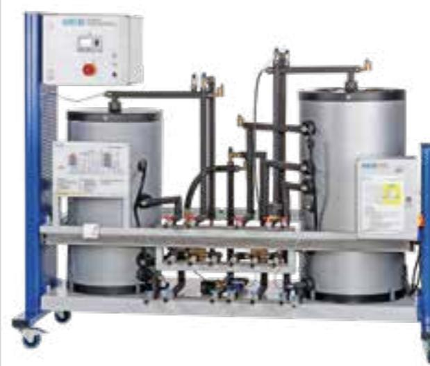
**HL 320.07****Underfloor heating / geothermal energy absorber**
