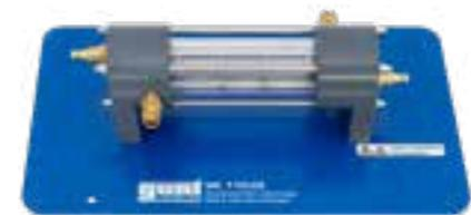
**WL 110.05****Finned tube heat exchanger** Heat transfer between water and air; cross-flow operation
