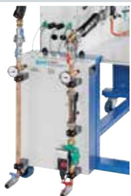
**ET 352****Vapour jet compressor in refrigeration**
