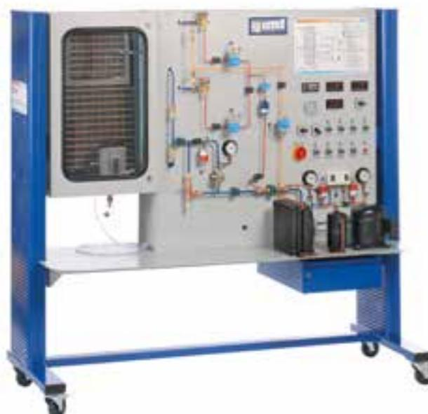
**ET 351C****Thermodynamics of the refrigeration circuit**
