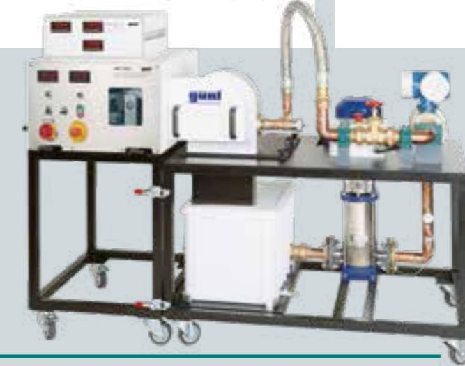
Trainer for turbines with Pelton turbine HM 365.31, supply unit HM 365.32 and brake unit HM 365
