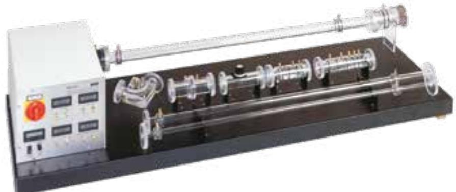
**HM 122****Pressure losses in pipes**
