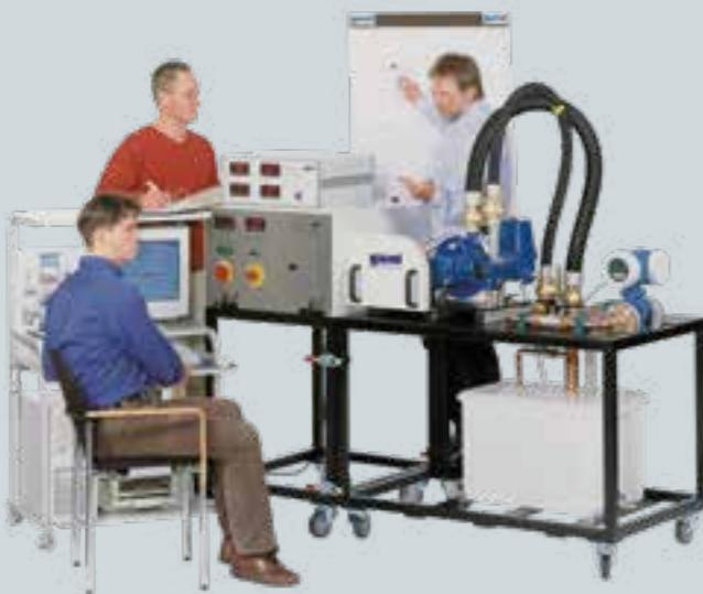
Trainer for positive displacement pumps with supply unit HM 365.10, piston pump HM 365.17 and drive unit HM 365
