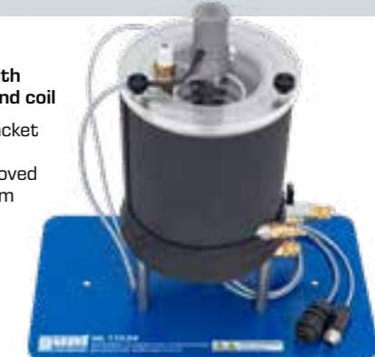
**WL 110.03****Shell & tube heat exchanger**
