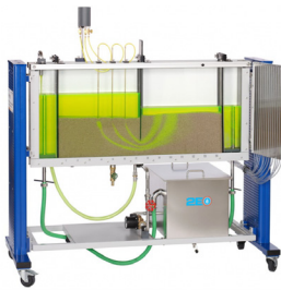
HM 169 - Visualisation of seepage flows
