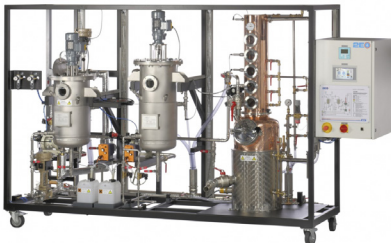
CE 640 - Biotechnical production of ethanol
