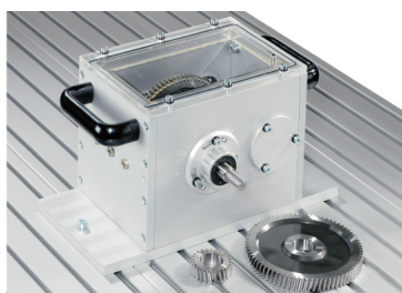
PT 500.15 - Damage to gears kit
