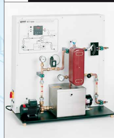
RT 644 Temperature Control Demonstration Unit
