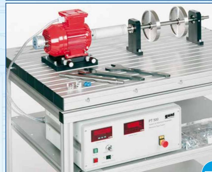
A range of training exercises relating to machinery diagnosis and monitoring can be carried out using just the PT 500 base unit together with the PT 500.02 instrumentation set.
