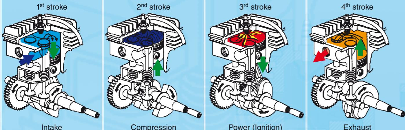
The piston moves from top dead centre to bottom dead centre. This takes in the fuel/air mixture.
