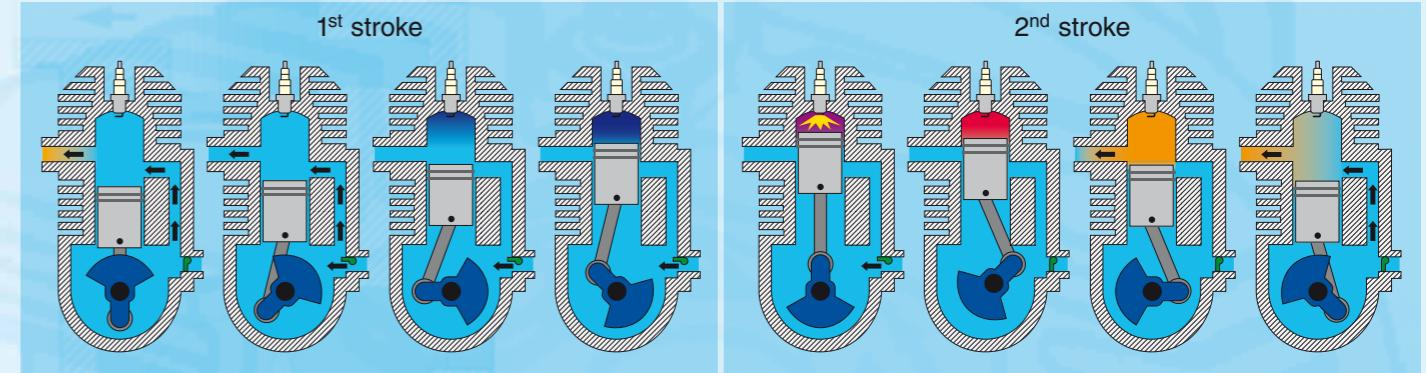
In the first stroke, the piston moves from bottom dead centre to top dead centre.
