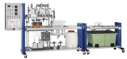
CE705- Activated Sludge Process
