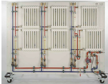
HL305 - Hydronic Balancing of Radiators
