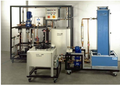
ET420 - Ice Stores in Refrigeration
