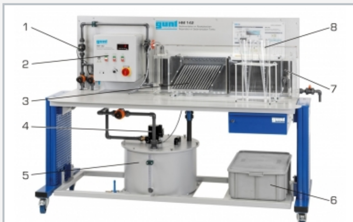
1 electromagnetic flow rate sensor, 2 switch box, 3 lamella unit, 4 pump, 5 suspension tank, 6 storage bin, 7 sedimentation tank with illumination, 8 Imhoff cone
