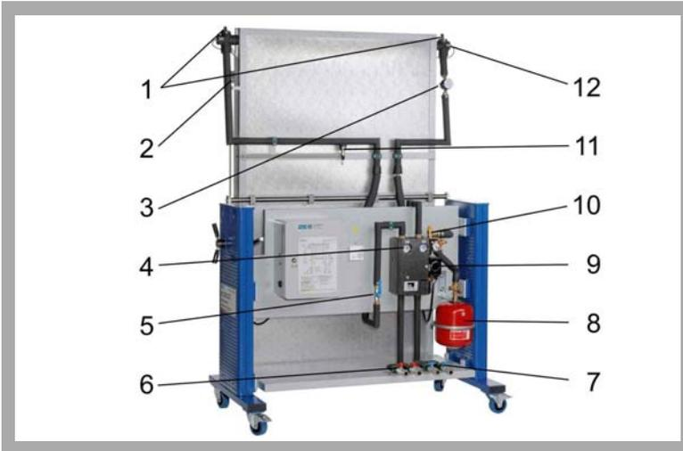
1 vent valves, 2 lighting sensor, 3 flow sensor, 4 thermometer collector outlet, 5 shut-off valve, 6 connectors for warm water, 7 connectors for cold water, 8 diaphragm expansion vessel, 9 circulation pump, 10 pressure relief valve, 11 pressure sensor, 12 temperature sensor
